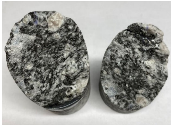
Tensile-induced rough Fracture
