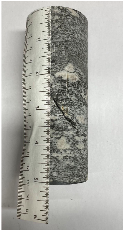
2-inch diameter sub-coring
